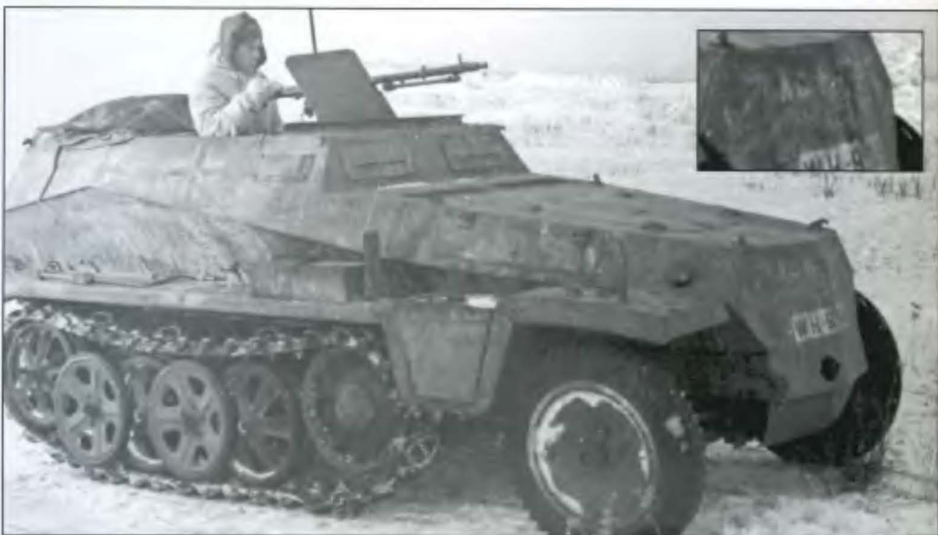
ABOVE: The left front wing is missing, as is the small axe, the wire cutters, front number plate and nose cap for the starter crank, but oddly, not the front dust shield. It has the second version intermediate height width indicators and the Fu. sprech. f. aerial is mounted on the right of the bodywork and not quite enough ice-cleats to place them in every third track plate. Generally lacking exterior stowage, this could be a rear echelon vehicle or headquarters vehicle and has either "A C F" or "A O F" on the nose above the front number plate.
