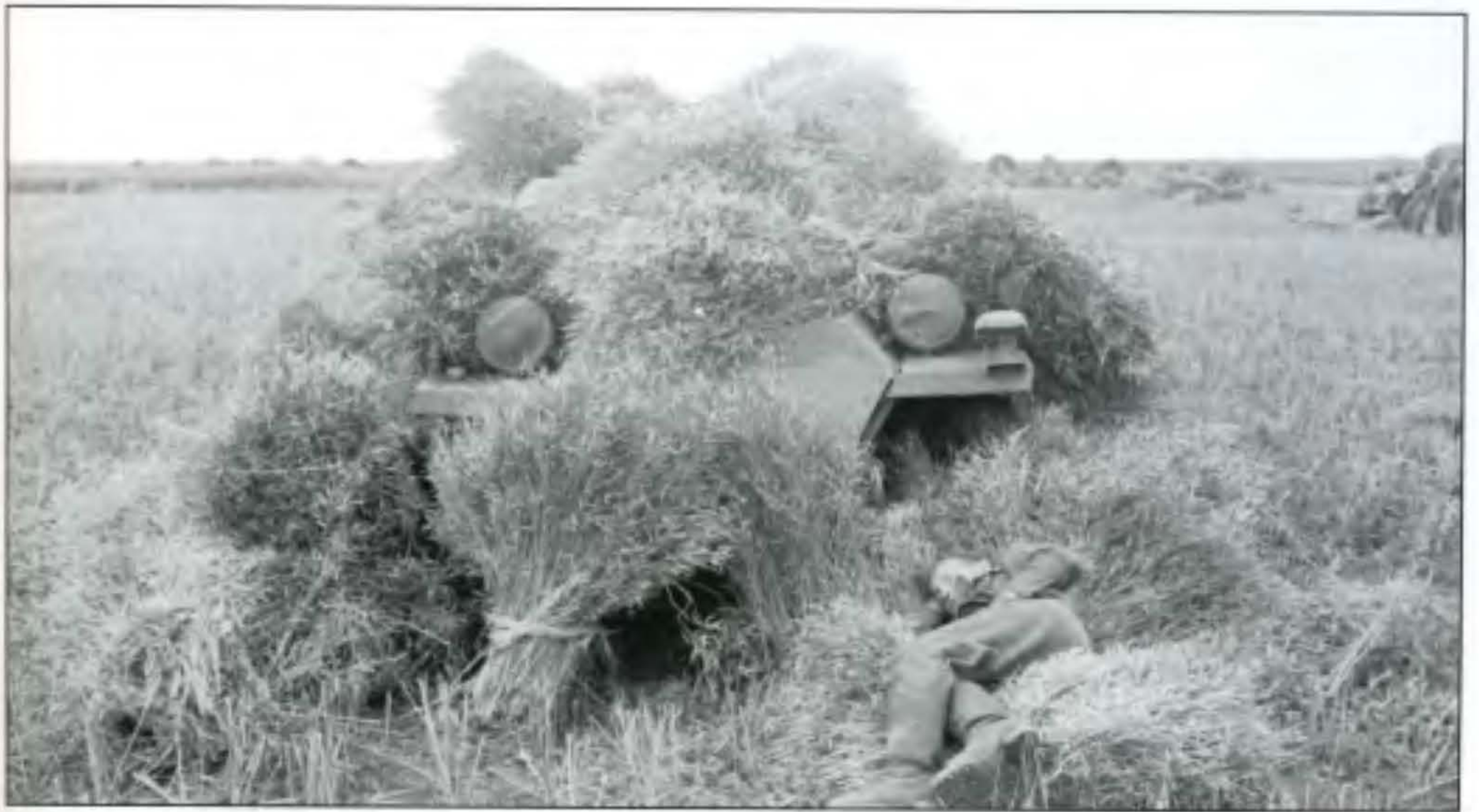
An almost mint example (except for the rear two stowage boxes) of an Sd Kfz 251/6 Ausf A complete with deployed aerial mast at the right rear corner. Note the extra front protection for the MG34 which is now on a raised mount, plus the use of a second shield at the rear. Just above and to the left of the Panzer Officer sitting alongside the 251 is what appears to be the divisional symbol for the 11th Pz. Division. The group of officers have settled down for what seems to be a relaxing few hours of lunch, whilst at least one Sd Kfz 250 crew member (above) grabs a few hours sleep amongst the sheaves of oats. The front of the Sd Kfz 251 shown opposite is just in shot to the right.
